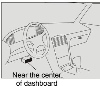
2. Plug the DBScar diagnostic connector into the vehicle's DLC;
