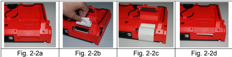
Fig. 2-2 Installing paper
